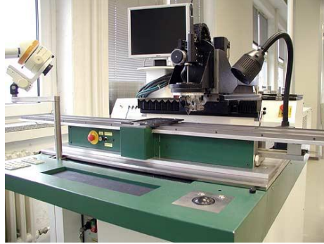
Fig 8. Semi-automatic wedge bonder to make aluminum wire bonds to the braised contacts.
