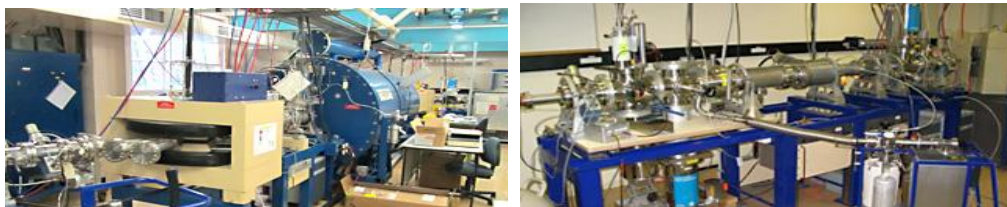
Fig 3. (left) Deep MeV implanter at the ANU. (right) Target chamber at the end of the beam line. The CVD plates were kept at liquid \text{N}_2 temperatures during implantation.
