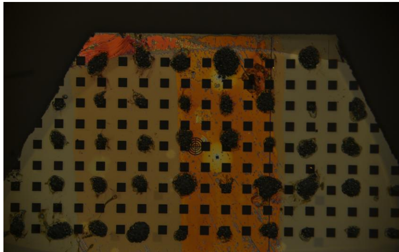
Fig 52. Optical microscopy image of electrical contacts to the H_2^+ implanted sample.
