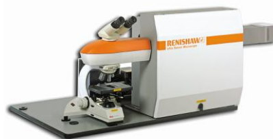
Fig 5. Renishaw InVia Reflex Raman spectrometer used to take the 532 nm Raman spectra presented. An infrared laser source was also used to avoid photoluminescence signals.
