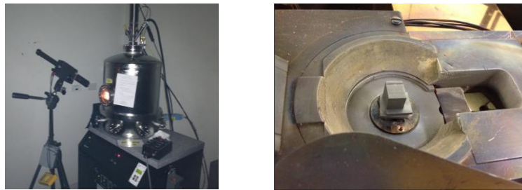
Fig 4. High temperature annealing of the diamond plate inside the Thermionics evaporator (left). Graphite box used for annealing mounted in the hearth of the e-gun evaporator (right).
