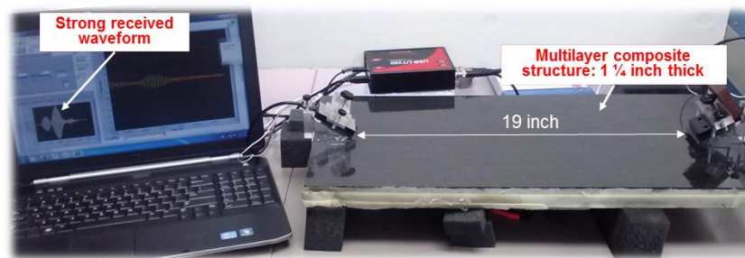
FIGURE 6. A portable ultrasonic scanning system was designed and tested successfully on multilayered structures including the ones with carbon fiber skin.
