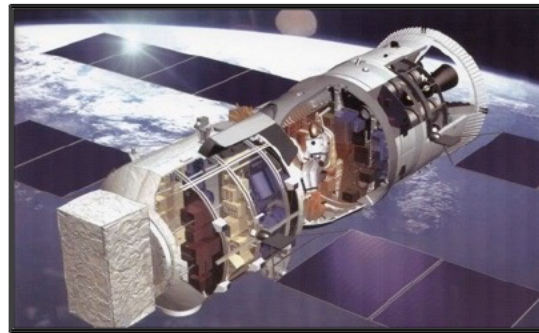
Figure 51: Shenzhou Spacecraft Cutaway
