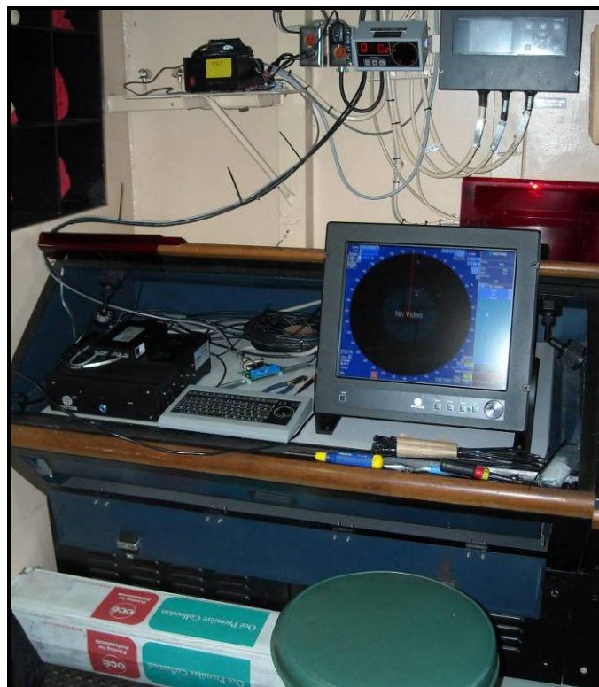
Figure A-2. Rutter Ice Navigation radar setup in the Chart Planning Station on the USCGC Healy.
