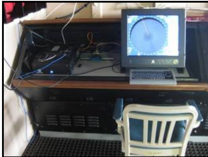
Figure 2. Setup of Rutter computer and radar display in the Chart Planning Station onboard the USCGC Healy.
