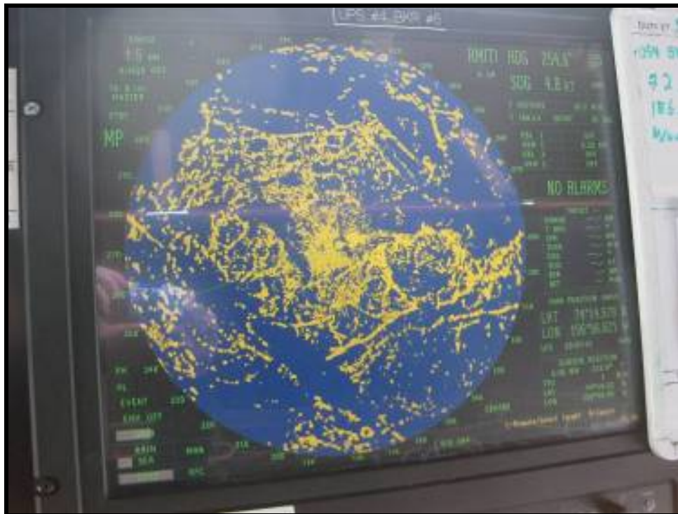
Figure 29. CG radar display while ship is stuck in an ice floe (1.5 nm range scale).
