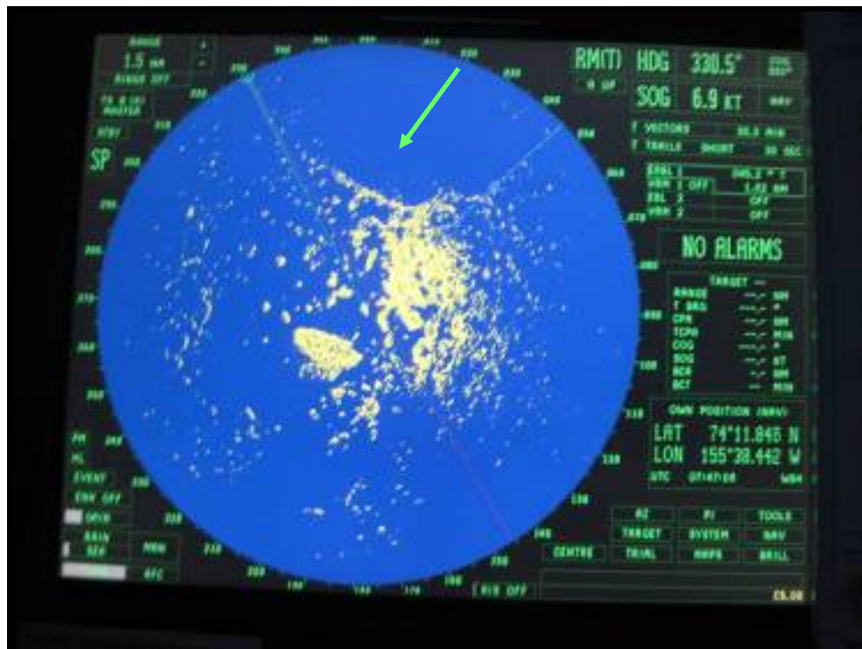
Figure 15. Arrow indicates lack of distinguishable ice field shown on CG radar 30 degrees east of the ship's heading and 0.5 nm away (1.5 nm range scale).
