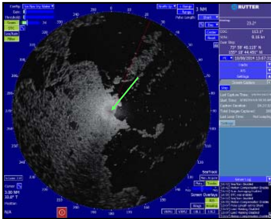
Figure 36. ASB clearing a path to open water (3 nm range scale; arrow indicates location of vessel heading roughly east).
