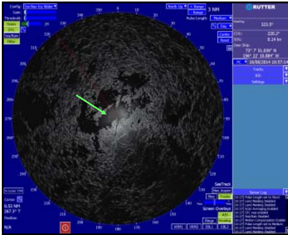
Figure 8. Ice Navigation radar screen capture during Stationary Procedure (3 nm range scale; arrow indicates location of a small ice chunk in an area of open water).
