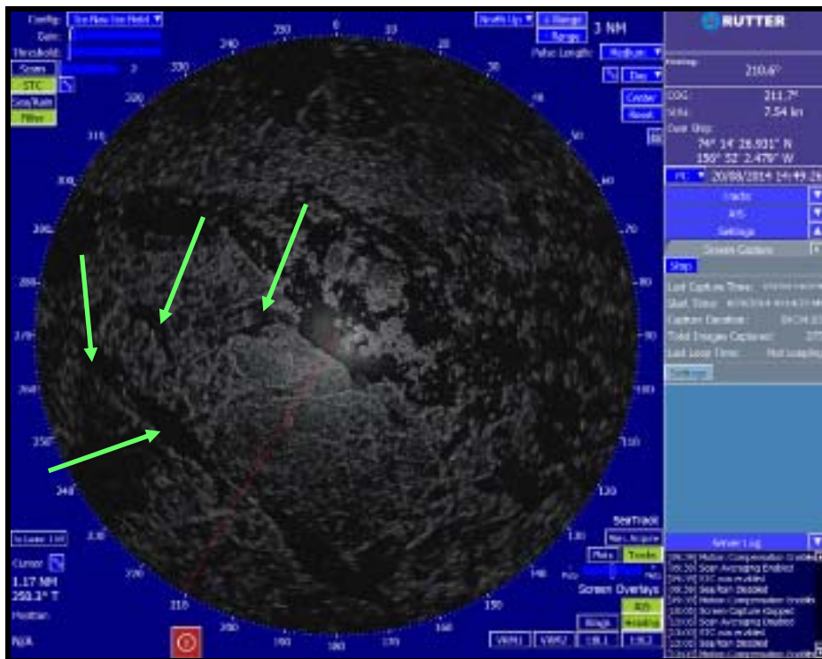
Figure 24. Upcoming ice floe that ship was stuck in; green arrows indicate the possible route ship could have taken; red line is ship's heading (3 nm range scale).
