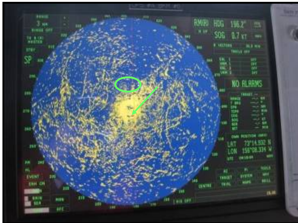
Figure 5. Photograph of Coast Guard radar display during Stationary Procedure (3 nm range scale; arrow indicates the patch of open water, which is difficult to discern on this display; circle suggests open water).
