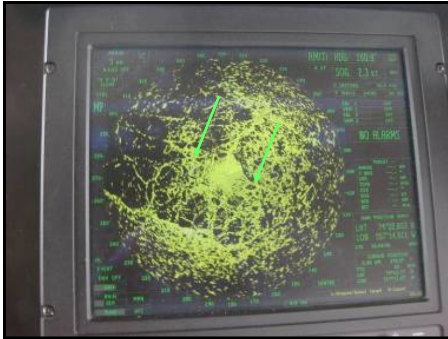
Figure 33. CG radar display of pressure ridge (3 nm range scale).
