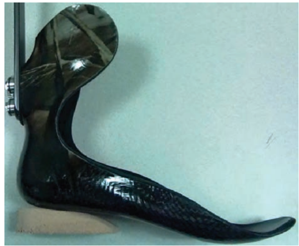
FIGURE 11 Current IDEO plantar surface design.
