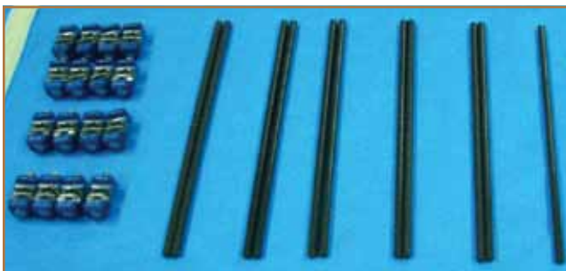
Figure 1. An inventory of the parts required for setup of the FEET is made, including 16 rod-to-rod coupling devices, and 11 carbon fiber rods (8x300 mm).
