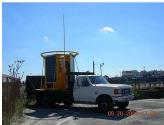
Figure 3: Bistatic transmitter with solar panels operating from the flatbed truck on beach at Sea Bright.
