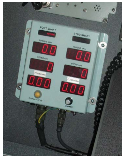
Figure 2 – Torsionmeter remote display unit, mounted in bridge on HMAS GLENELG
