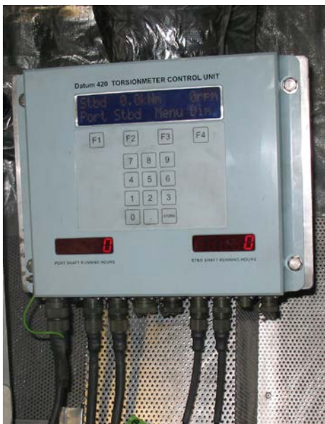
Figure 1 – Torsionmeter control unit, mounted in engine room on HMAS GLENELG.
