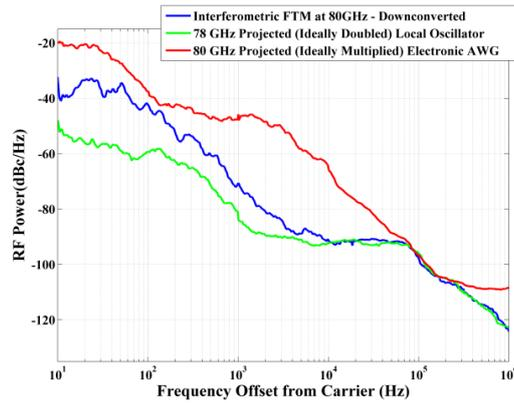
**Fig. 4.** Phase-noise comparison of 80 GHz continuous waveform (generated using photonic-assisted interferometric RF-AWG and down-converted with an LO at  $2 \times 39$  GHz = 78 GHz), expected (projected) 78 GHz local oscillator phase-noise, and a 5 GHz signal from an electrical arbitrary waveform generator ideally multiplied to 80 GHz.
