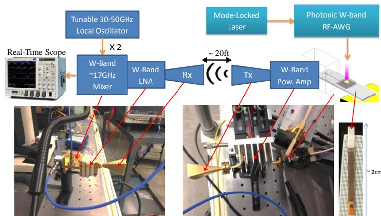
Fig. 1. The system setup for our MMW arbitrary waveform generation at W-band.
