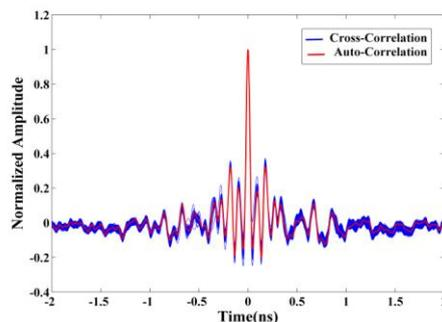
**Fig. 3.** Cross-correlations between a reference chirped waveform and 4000 consecutive linear down-chirp waveforms (in blue) and autocorrelation of the reference down-chirp waveform (in red).
