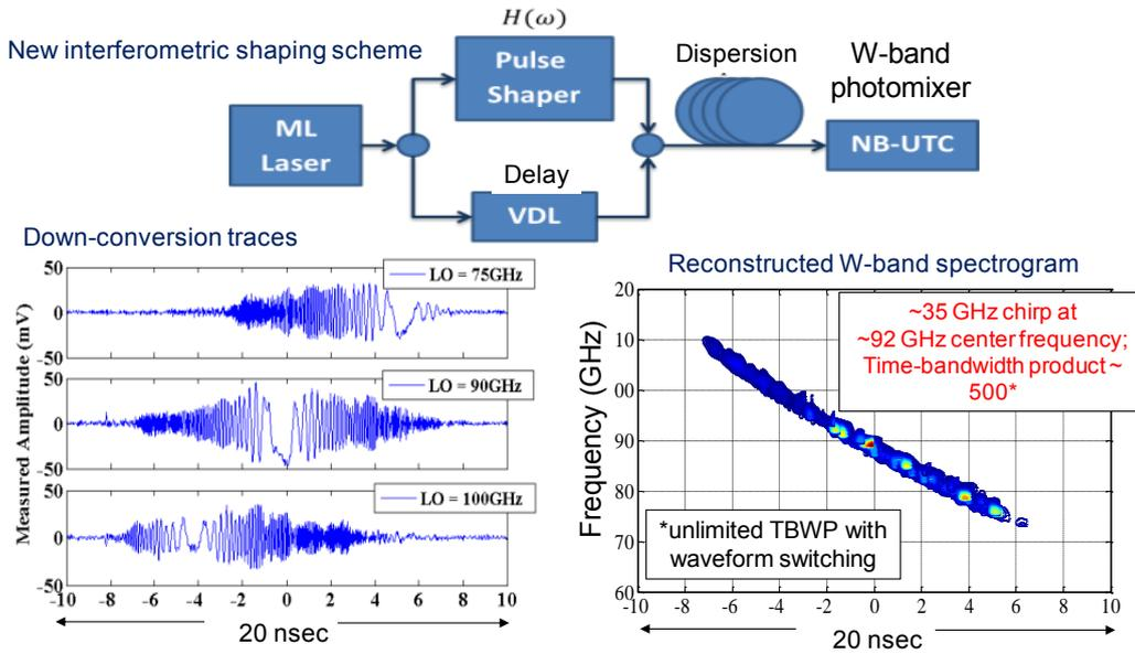
Fig. 2. The waveform of generated MMW chirp pulse
