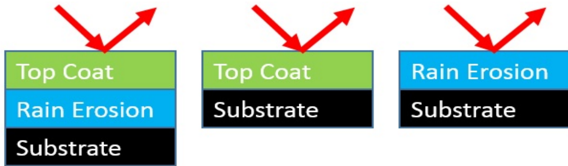
Figure 30. If the top coat is the only layer responsible for the reflectance spectra then the first and second samples should have identical reflectance spectra. If the first and second spectra are distinct the third sample will provide information on the reflectance spectra of the middle layer and later assist in determining of the substrate contributes to the reflectance spectra.
