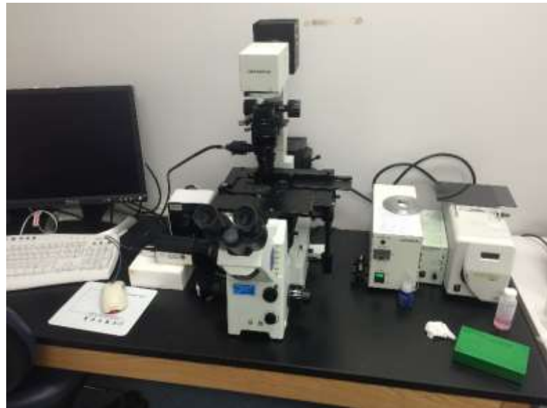
Figure 8. CytoViva Dual Mode Fluorescence System, AFRL, 711th HPW.
