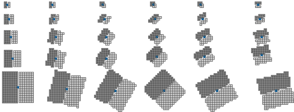
Figure 18. The Haar wavelet masks are predefined for all possible scales and rotations at 15 degree increments. The far left column shows the Haar wavelets used in upright SURF which can be calculated much more quickly using integral images. For features with orientation, each pixel in the Haar wavelet mask must be accessed to calculate the response, leading to dramatically increased processing time for larger scale features.
