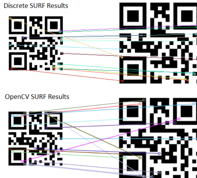
Figure 32. The fifteen best matches by the Discrete SURF algorithm (top) are directly compared to the matches found by the OpenCV SURF (bottom) implementation for 150% scaled images.
