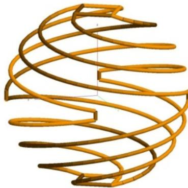
**Figure 59 The Folded Multi-arm Spherical Helix (FMSH)**
