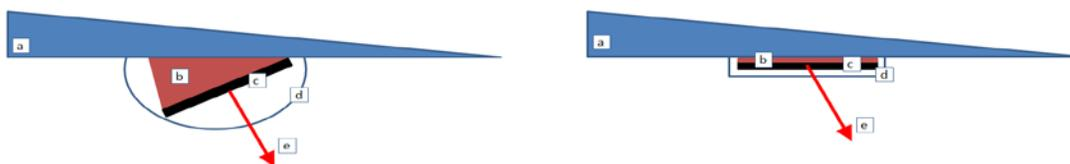
**Figure 16 (a) Traditional High-Gain Antenna in a Pod; (b) Low Profile Antenna in a Pod with a. Platform, b. Pedestal, c. High Gain Antenna, d. Radome, e. the Direction of the Main Beam**
