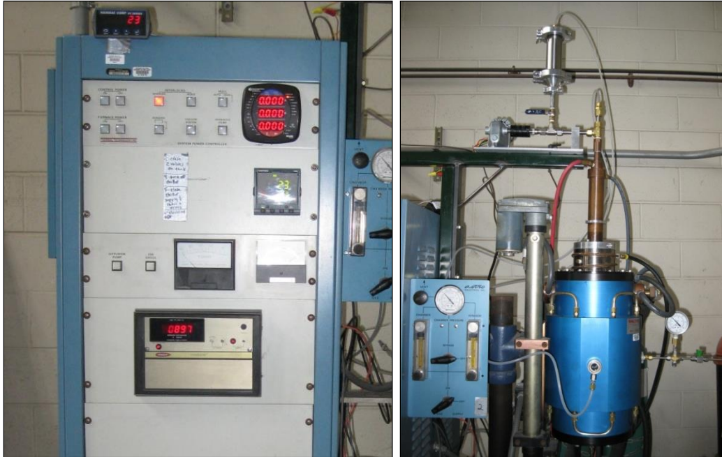
Fig. 2.3 Rapid carbothermic reduction furnace with Cu cold finger and screw feed
