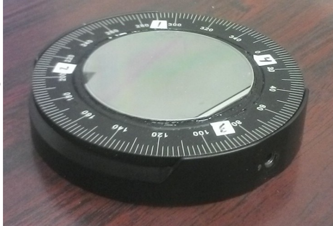
Figure 69: A polarizer based FPI mirror. Using glue, the polarizer is attached so it protrudes from the front surface of the rotation stage.
