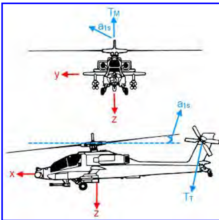
Figure 1. Coordinate frame and forces acting on a helicopter
