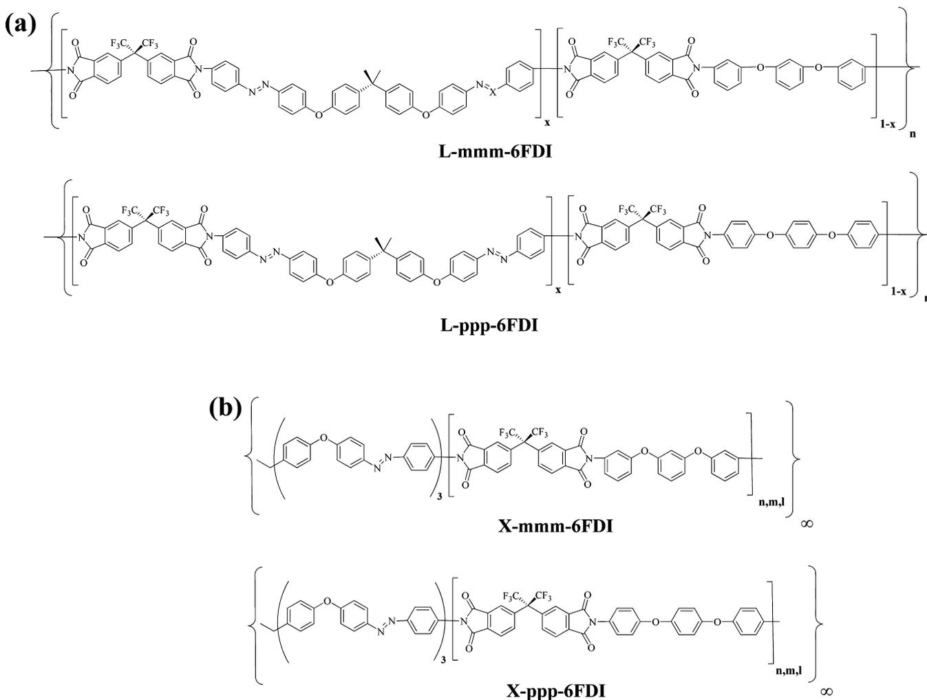
Figure 1. Chemical structures of (a) linear polyimides and (b) cross-linked polyimides.
