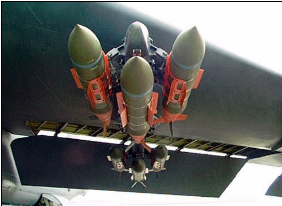
Figure 2-17: Multiple Ejector Rack Loaded Up with Three Air-to-Ground Munitions [19].
