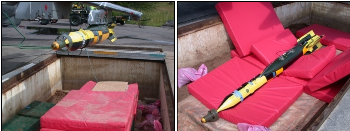
Figure 4-27: Static Ejection Test.
