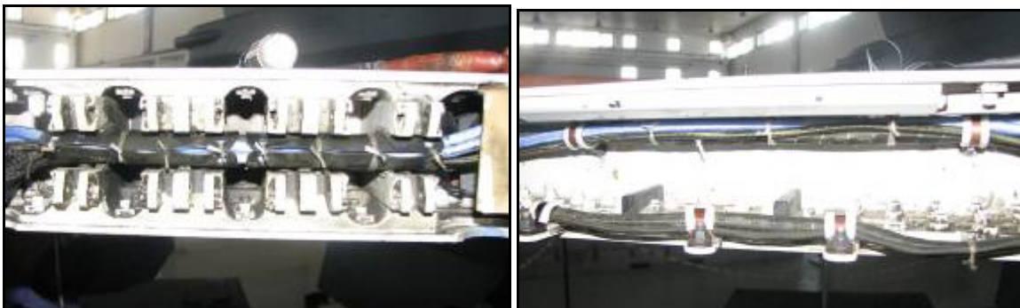
Figure 4-44: Flight Test Instrumentation Cabling on F-16 Wings.
