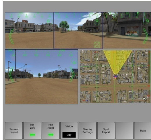
Fig. 1. Vehicle Commander (VC) Warfighter-Machine Interface (WMI), consisting of a 180° field-of-view banner across the top, a 60° field-of-view window on the left hand side, and an overhead map on the right hand side.
