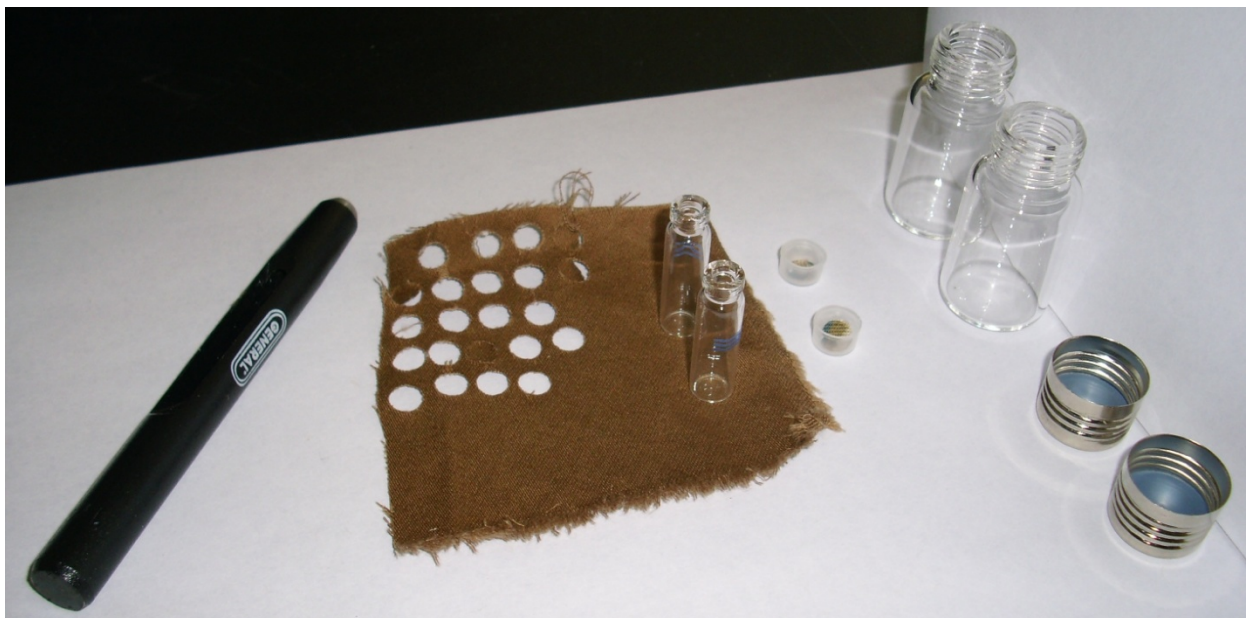
Figure 6: Photo of the hole punch, fabric, small inner vials, modified caps, headspace vials, and headspace vial caps used for the preparation of vial-in-vial permeation test samples.
