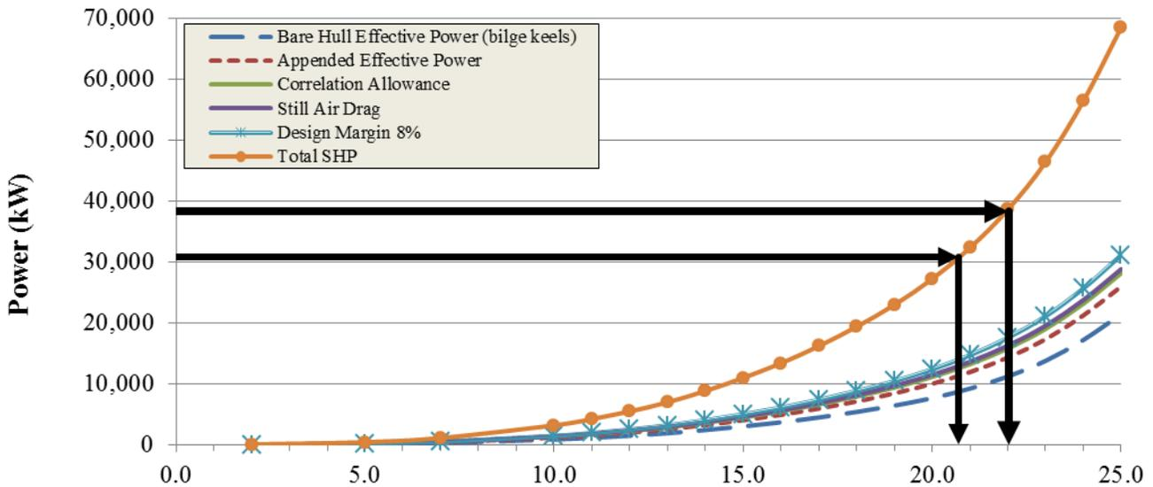
**Figure 6: HSR(R) Speed-Power Curve**
