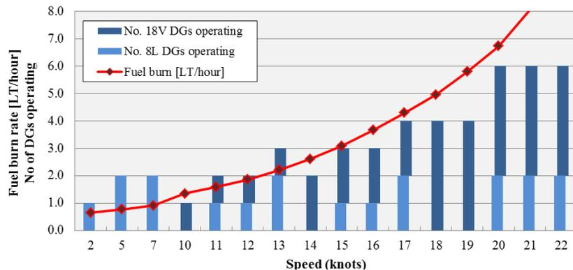
Figure 8: Hourly Fuel Burn (cruise ship service load)
