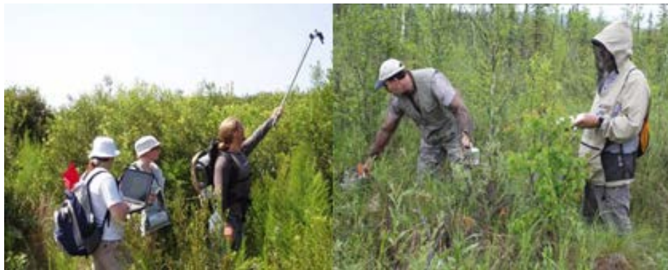
Figure 6. Canopy spectral reflectance collection ( left ) and leaf-level IRGA ( right ) at FL2 and CR sites.
