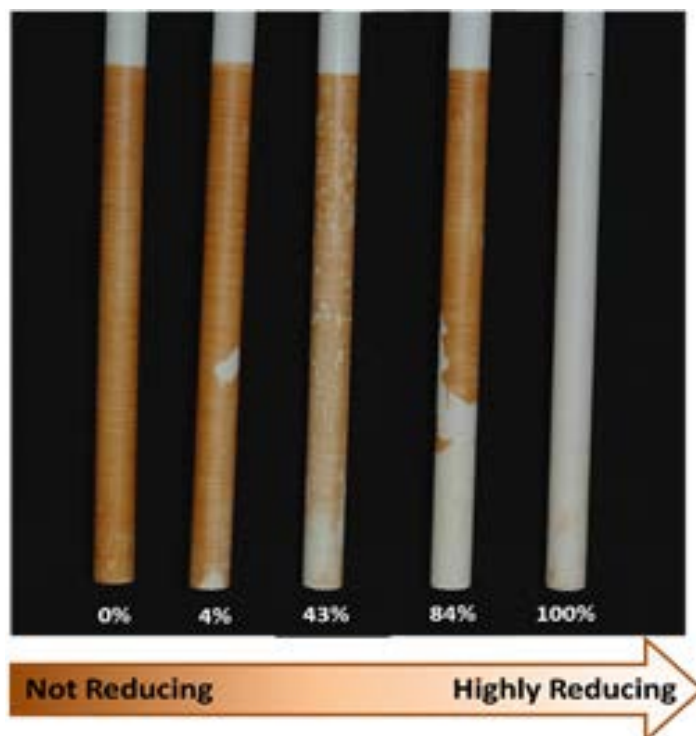
Figure 11. Example IRIS tubes with varying degrees of iron reduction.
