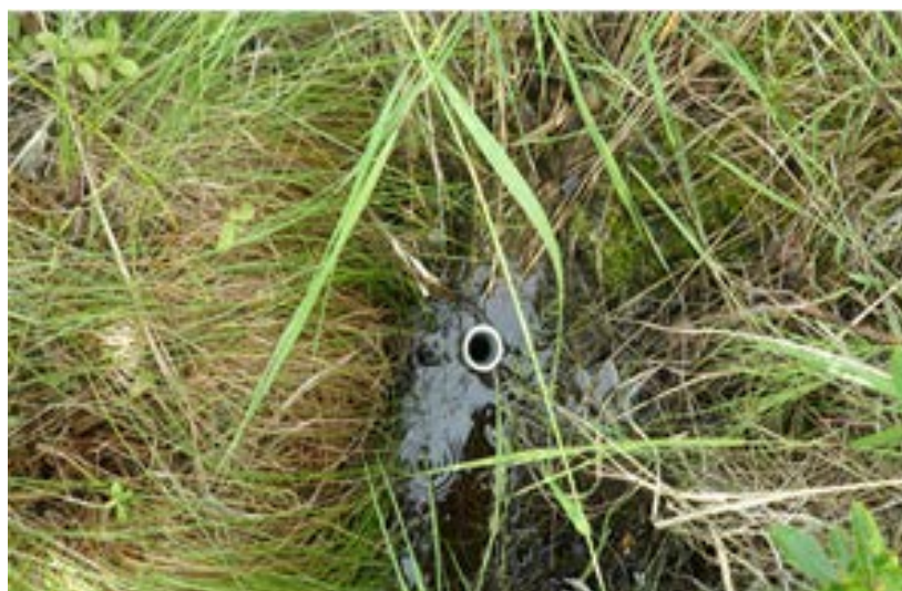
Figure 4. The sample area in between tussock sedges where pH and Eh were measured (white PVC pipe).
