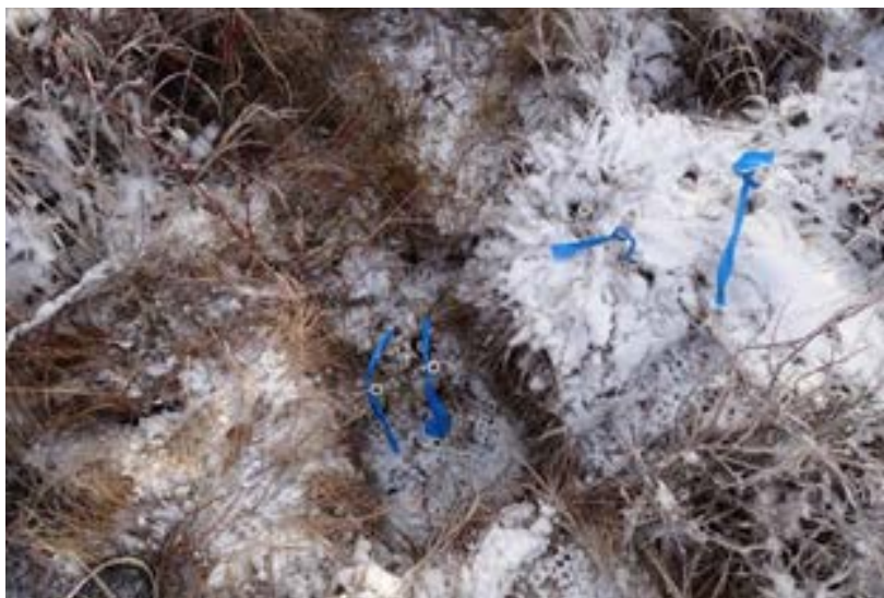
Figure 5. Nested IRIS tubes installed at the FL2 site in the tussock sedges and in the regions between the tussocks.
