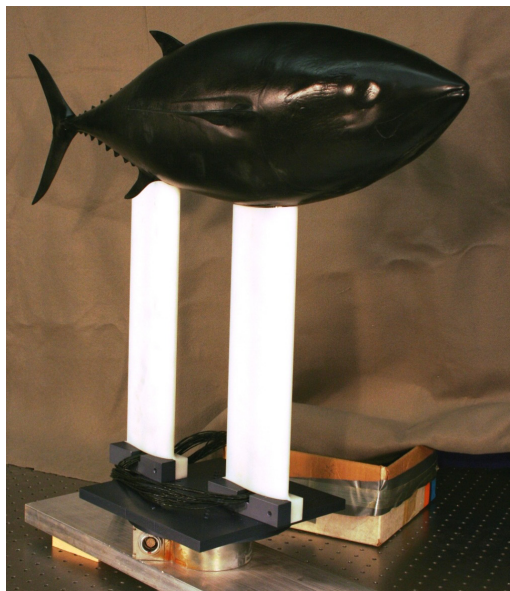
Figure 4. Tuna Model Showing Fairings, Angle-Indexing Plate, and Load Cell
