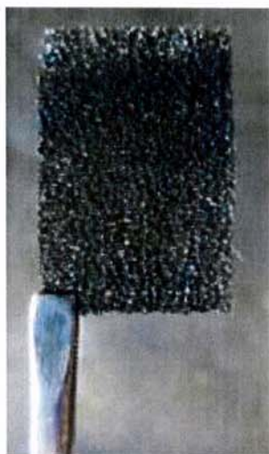
FIGURE 36: EXAMPLE OF \text{MnO}_2 GRADIENT AFTER ELECTRODEPOSITION ONTO A PU SPONGE.
