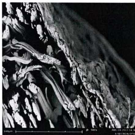
FIGURE 54: CROSS-SECTIONAL SEM OF PA6 WINGED FIBER WITH CNT AND \text{MnO}_2 .
