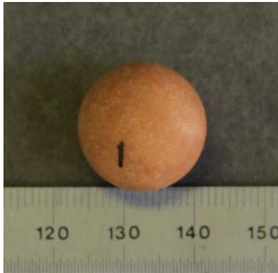
FIGURE C-4. Spherical CompB Sample (mm Scale).
