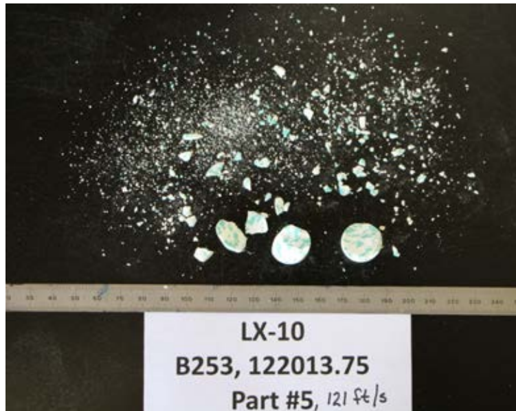
FIGURE 8. Cylindrical LX-10 Sample Impact Damaged at 121 ft/s.
