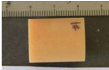
FIGURE C-3. Typical CompB Friability Sample (mm Scale Divisions).
