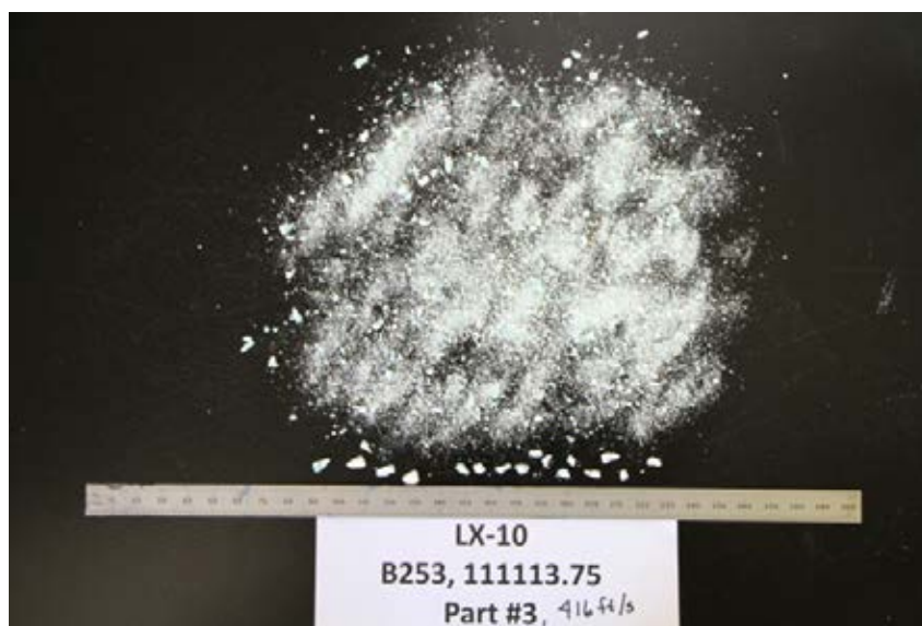
FIGURE 19. Spherical LX-10 Sample Impact Damaged at 416 ft/s.
