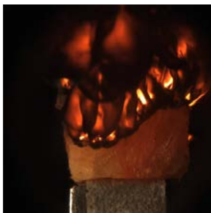
FIGURE C-29. TNT Burning Sample at 10.34 MPa (1,500 psia).
