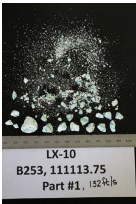
FIGURE 15. Spherical LX-10 Sample Impact Damaged at 132 ft/s.
