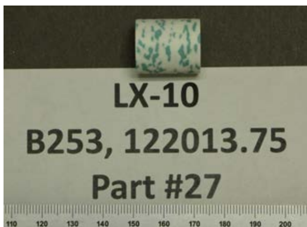
FIGURE C-5. Typical Cylindrical CompB Friability Sample (mm Scale Divisions).
