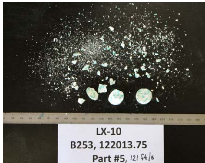
FIGURE C-11. Cylindrical LX-10 Sample Impact Damaged at 121 ft/s.
