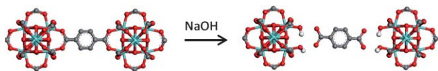
Scheme 2 Proposed mechanism for the structural breakdown of ZrMOFs in the presence of NaOH. Carbon (gray), hydrogen (white), oxygen (red), and zirconium (light blue) atoms can be seen; hydrogen atoms are omitted for clarity.
