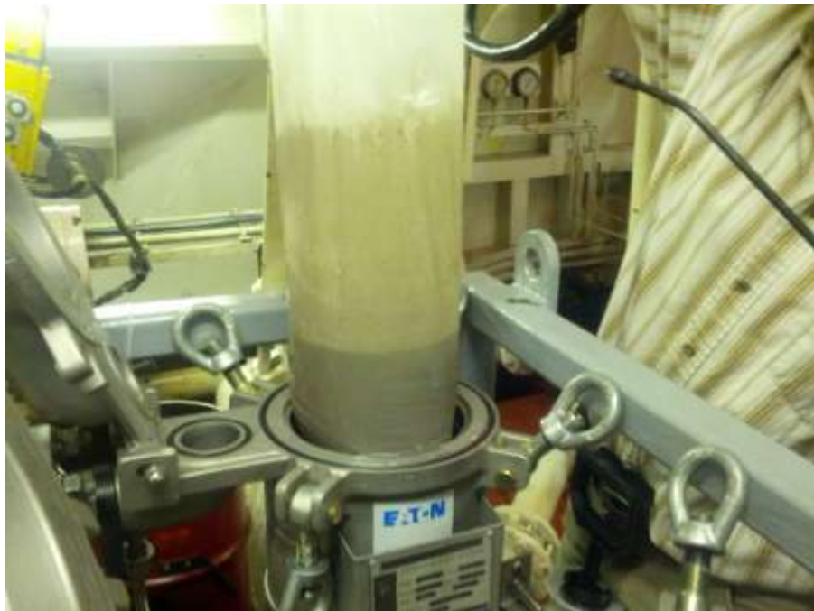
Figure 7. Full p3SFS filter bag after completion of a sampling event.
