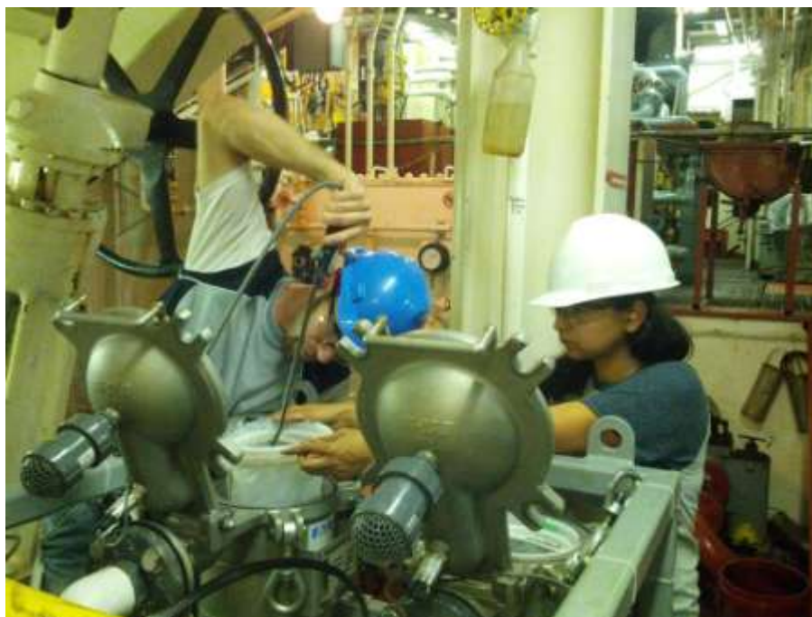
Figure 8. GSI sample collection team rinsing the inside of the p3SFS filter bag.
