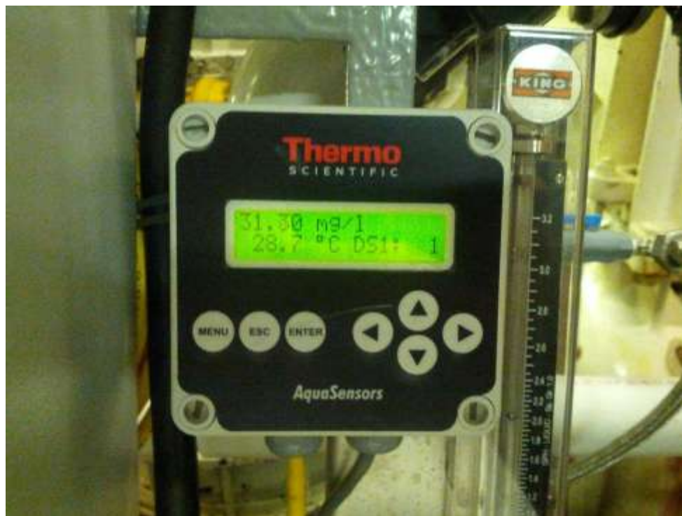
Figure 32. AquaSensors display on the p3SFS showing the in-line temperature and turbidity data in real time.
