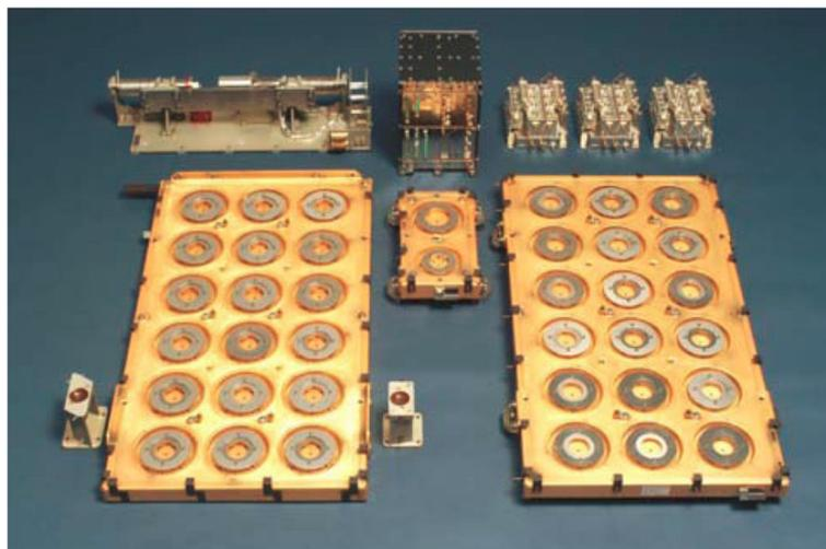
**Figure 6** Image of the GRAS instrument flown on MetOp-A. Images showing the GRAS instrument with both occultation antennas (front left and front right), the Zenith antenna (front middle) and the R/F front ends and main electronics unit (in the back).
