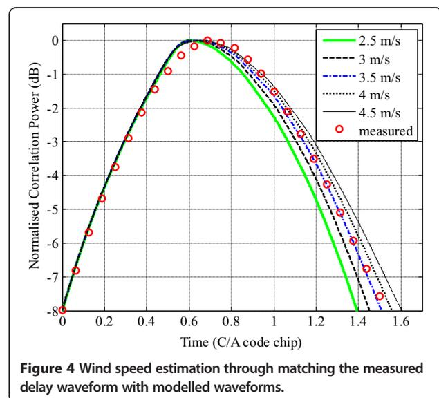
**Figure 4** Wind speed estimation through matching the measured delay waveform with modelled waveforms.
