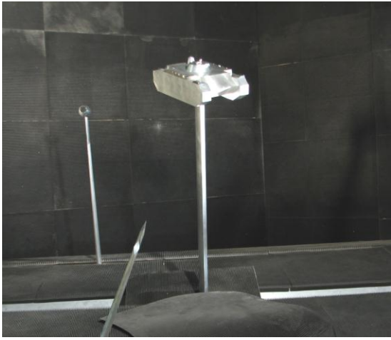
Figure 3. Front-View of Target Positioning System with Calibration Pylon at the Rear (Left), Target Pylon with Adjustable Elevation and Target Azimuth (Center), and In-Scene Calibration Pylon with Dihedron (Lower-Left)
