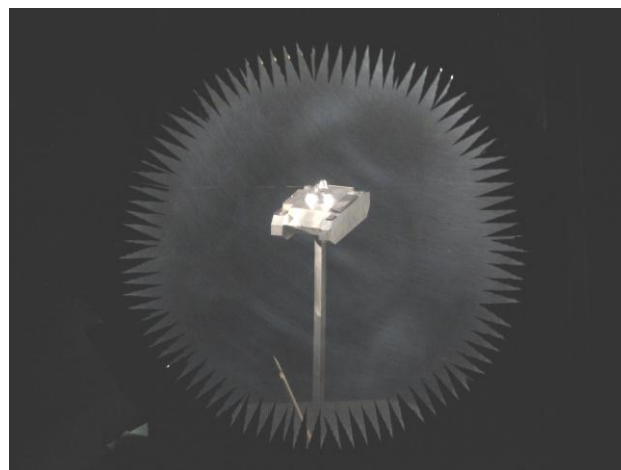
Figure 2. Primary (Antenna) Mirror in Compact Range with RAM Edge Treatment Showing the Reflection of the Complex Target Simulator and In-Scene Dihedron
