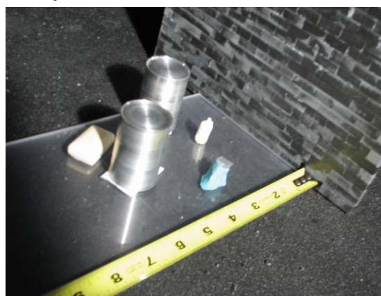
Figure 9. Scale-Model Scene for Preliminary Demonstration of Scale-Model Through-Wall Imaging
