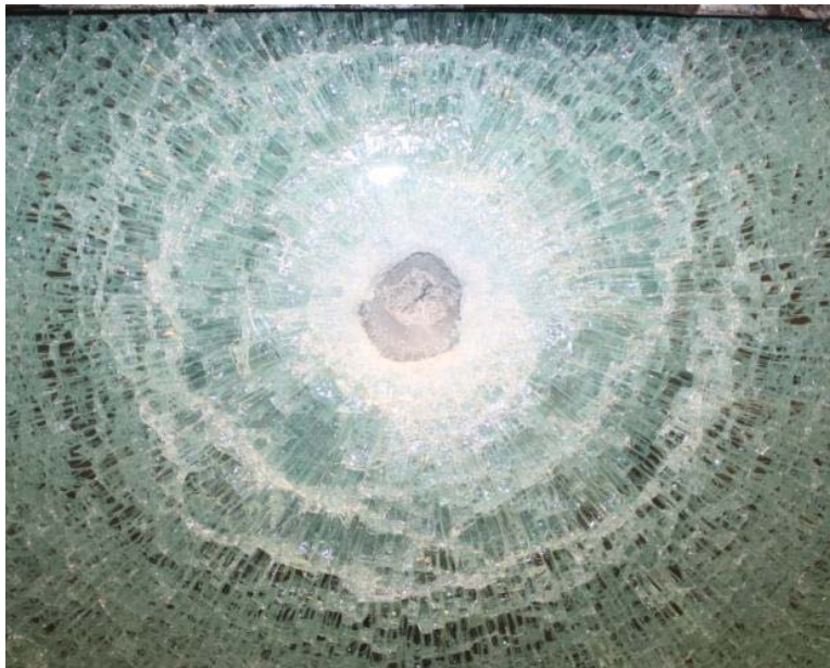
Figure 1. Typical Response of a Tempered Glass Laminate to a Single High Velocity Impact by a Small Arms Rifle Projectile
