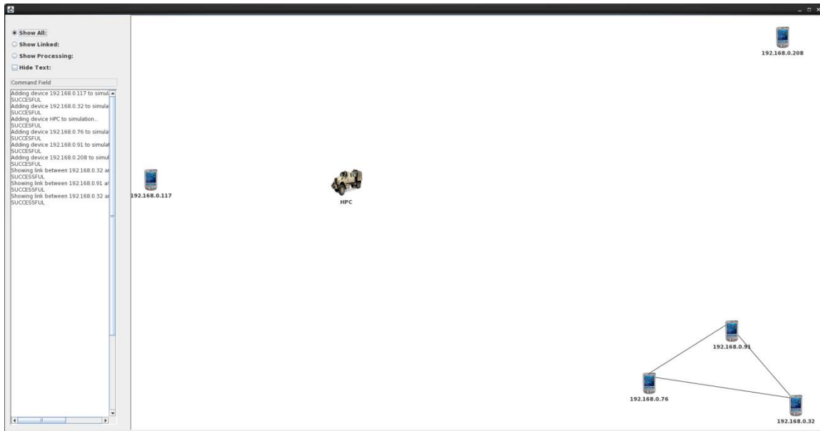
Fig. 9 Sample output of the visualization system. In this scenario, there are 5 mobile devices and one mobile HPC, and there is network connectivity between the 3 devices in the lower right corner.
