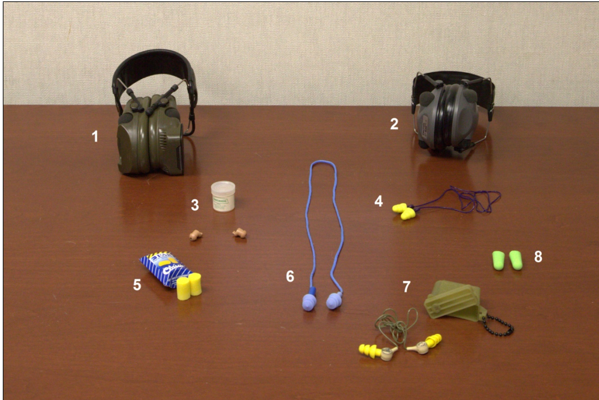
Fig. 5 ARL photo of examples of hearing protection devices including 1) Peltor supra-aural hearing protection, model MT15H68FB-03, 2) Peltor Tactical 6-S supra-aural hearing protection, 3) Gunfenders, 4) Ear Ultrafit, 5) Ear Classic foam earplugs, 6) Tasco Tri-fit, 7) Combat Arms Earplugs generation 2, and 8) Moldex Pura-fit 6800.
