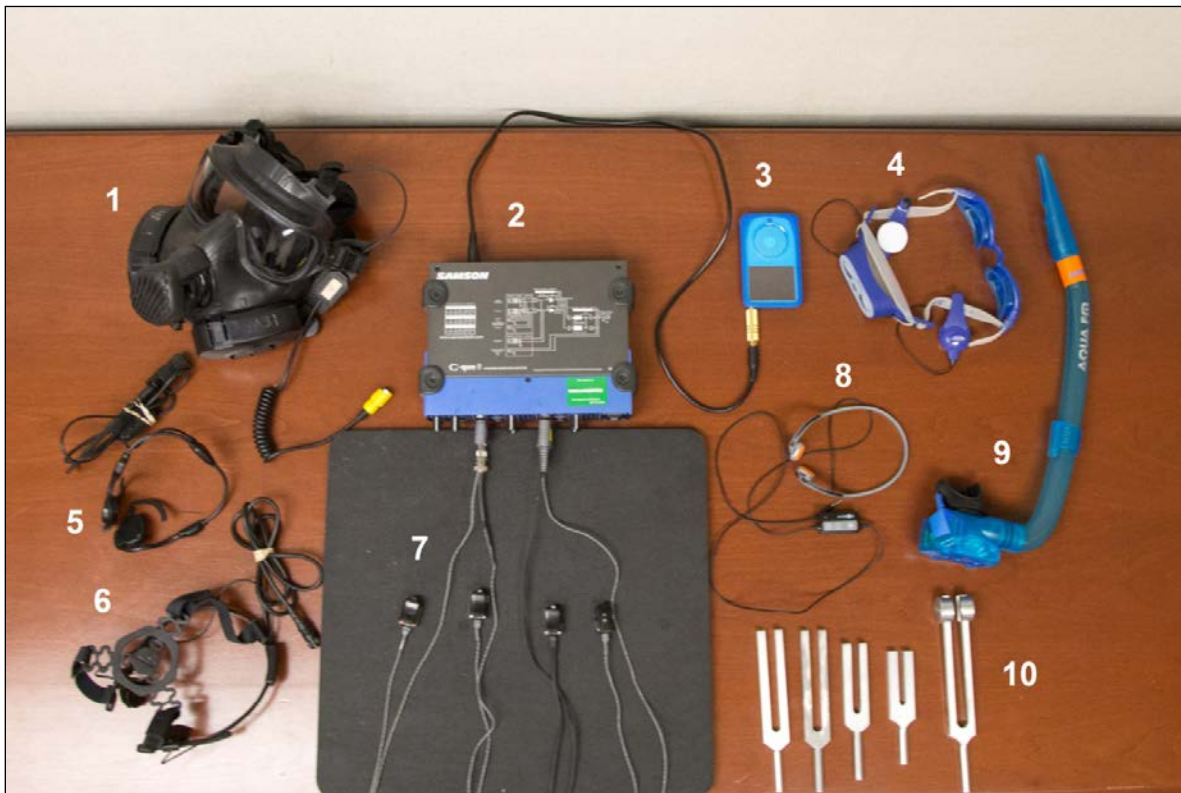
Fig. 14 ARL photo of the bone conduction station including 1) full-face respirator with Huari HRE-5673 system, 2) Samson C-que 8-headphone amplifier, 3) iPod, 4) Finis SwiMP3, 5) Goldendance Double Bone, 6) Temco HG-17, 7) Radioear B70A bone vibrators, 8) Aftershokz Sport headset, 9) Amficom Aqua FM, and 10) tuning forks.
