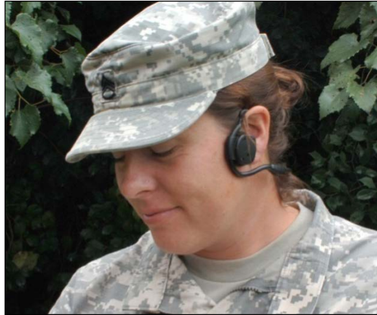
Fig. 13 ARL photo of a Soldier wearing a bone conduction communication headset. The ears are left unoccluded to maximize situation awareness.
