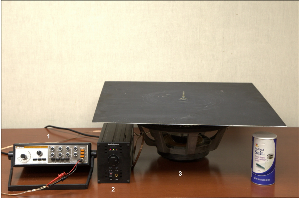
Fig. 10 ARL photo of Chladni plate station setup including 1) function generator, 2) audio amplifier, and 3) plate and loudspeaker assembly.
