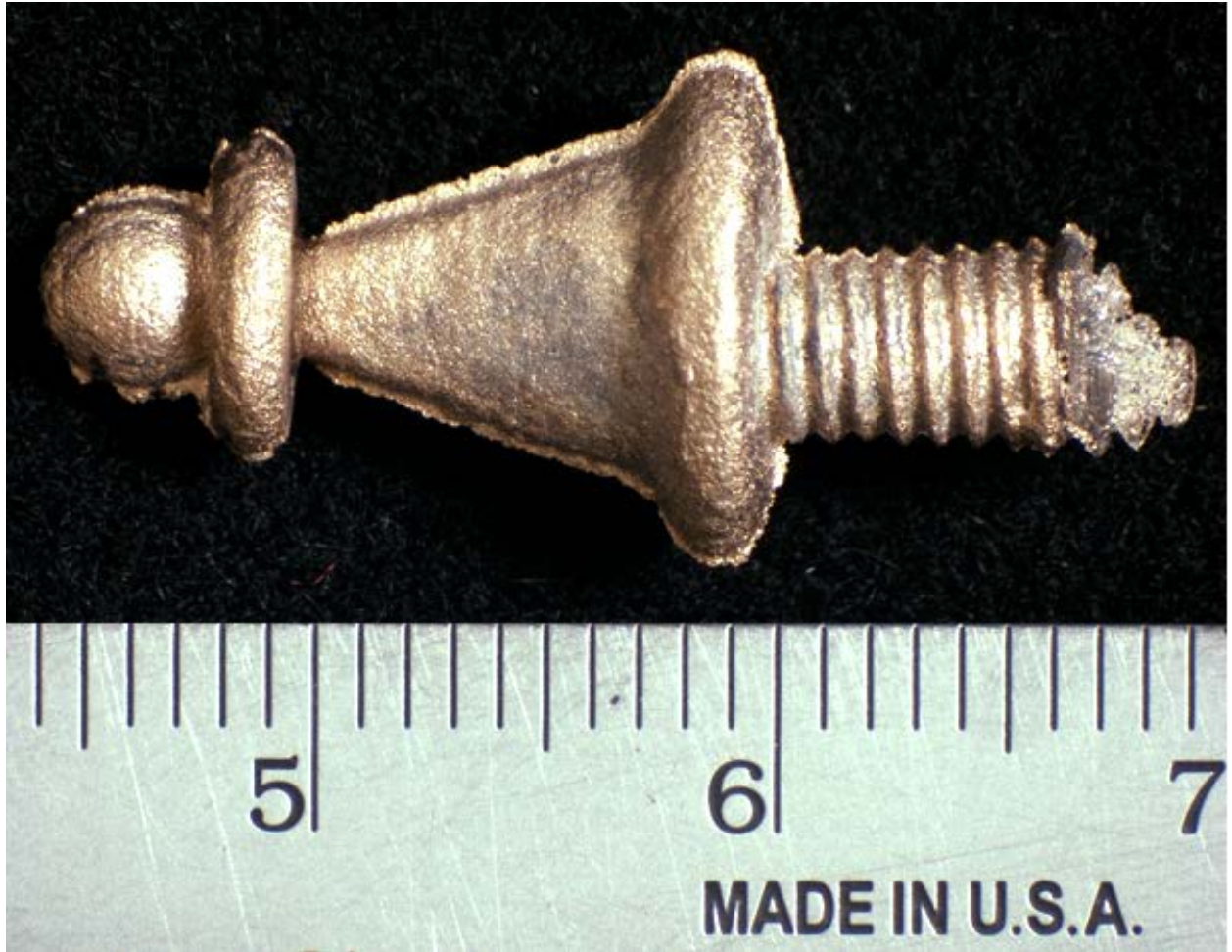
Fig. 6 The ease of processing allows for complex parts to be created. This “pawn” was made by filling a 2-piece mold with the Cu alloy powder and applying pressure at one end with a machine screw. The detail of the mold was reproduced with significant accuracy (scale in centimeters).
