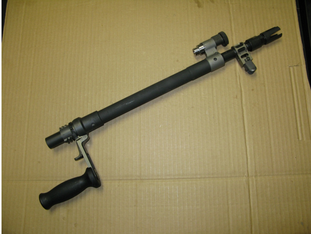
Fig. 5 Finished niobium-lined M240 machine gun barrel with flash suppressor attached
