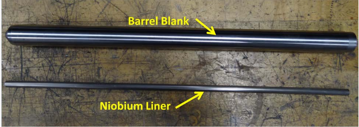
Fig. 2 Gun tube and niobium-liner hardware
