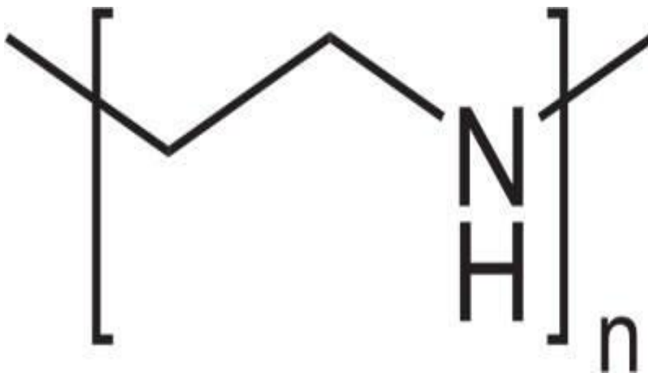
Figure 3-1. Structure of Linear Polyethyleneimine
