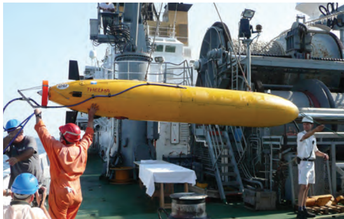
Figure 4-2: The NURC OEX- Harpo AUV used during GLINT '10. This AUV communicates with the ship and the MIT Unicorn AUV via acoustic communication (underwater). It also carries a GPS for positioning.
