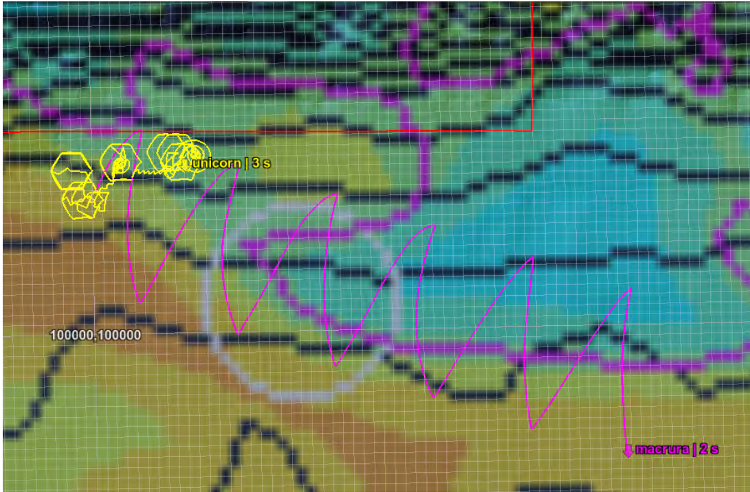
Figure 5-13: An adaptive 2D front tracking mission with poor front tracking at constant depth. The adaptive AUV path is the yellow ‘ Unicorn ’ line and the preplanned AUV path is the magenta ‘ Macrura ’ line, while the frontal isotherm location is highlighted (at the time of this snapshot) by the blurry purple line.
