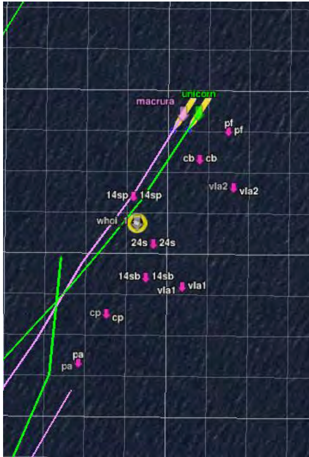
Figure 3-5: The Google Earth interface for Ocean Vehicles (GEOV) [63] real-time topside situation display in Google Earth [64] showing two AUVs swimming in sync (trailed by purple and green lines) past an acoustic communications buoy (yellow circle) and a field of objects on the sea floor (pink arrows).
