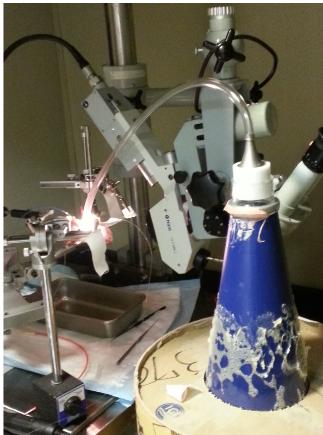
Figure 5: Temporal bone as mounted with LDV and manipulator. Note micrometer stage used to advance pressure probe into scala.
