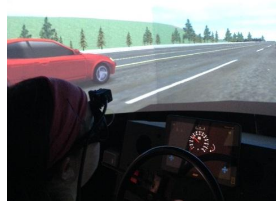
Driver wearing eye tracking glasses while performing the Operational Peripheral Vision Test
