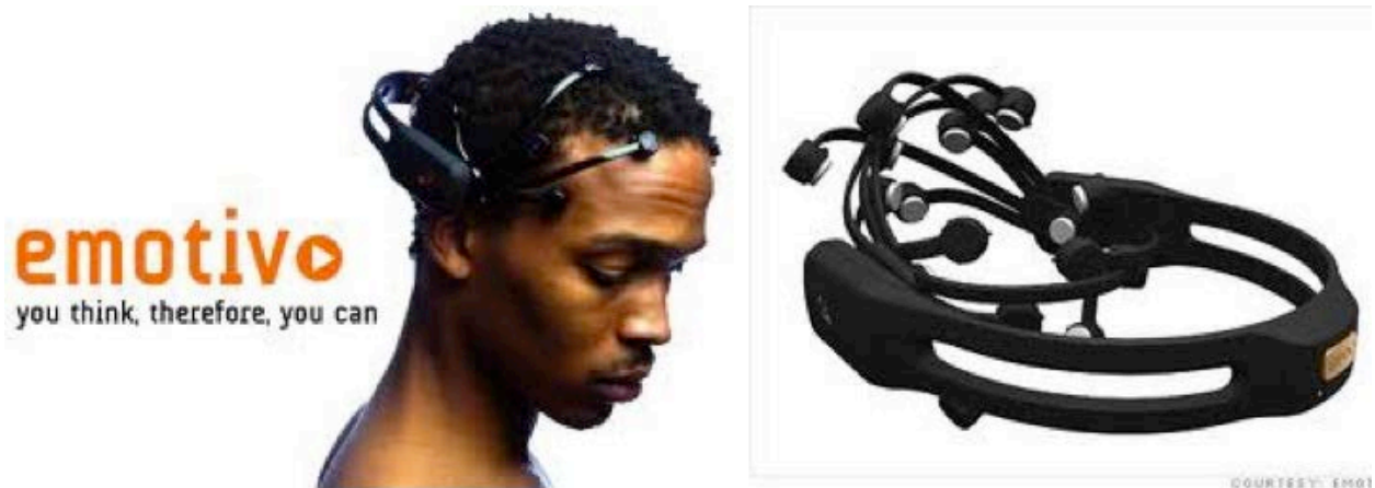
Figure 13. Emotiv's EEG electrode headset that we are using as a model for visual cortex electrode headset and flexible placement of electrodes for VEP measurements of regional visual field defects.
