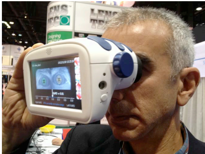
Figure 2: New portable hand-held binocular pupillometer prototype instrument that was developed by Neuroptics Inc, based on our suggestions. This new pupillometer can deliver
