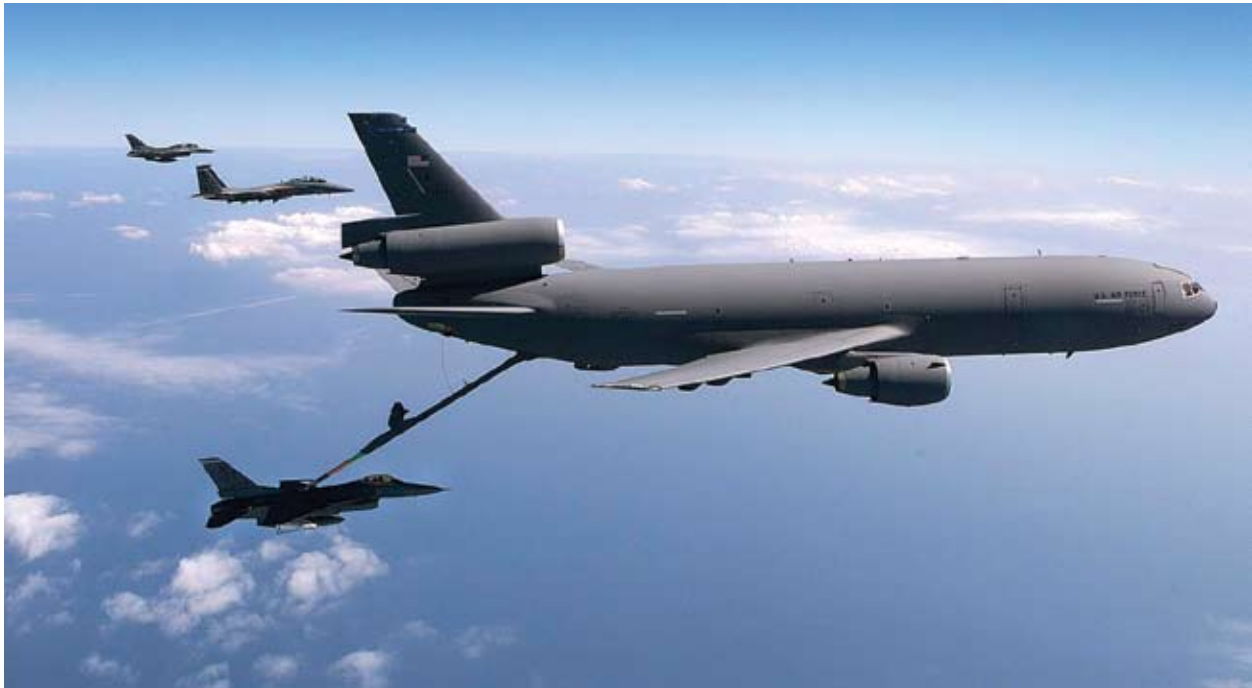
Figure 55. A KC-10 refueling an F-16. (USAF photo)
