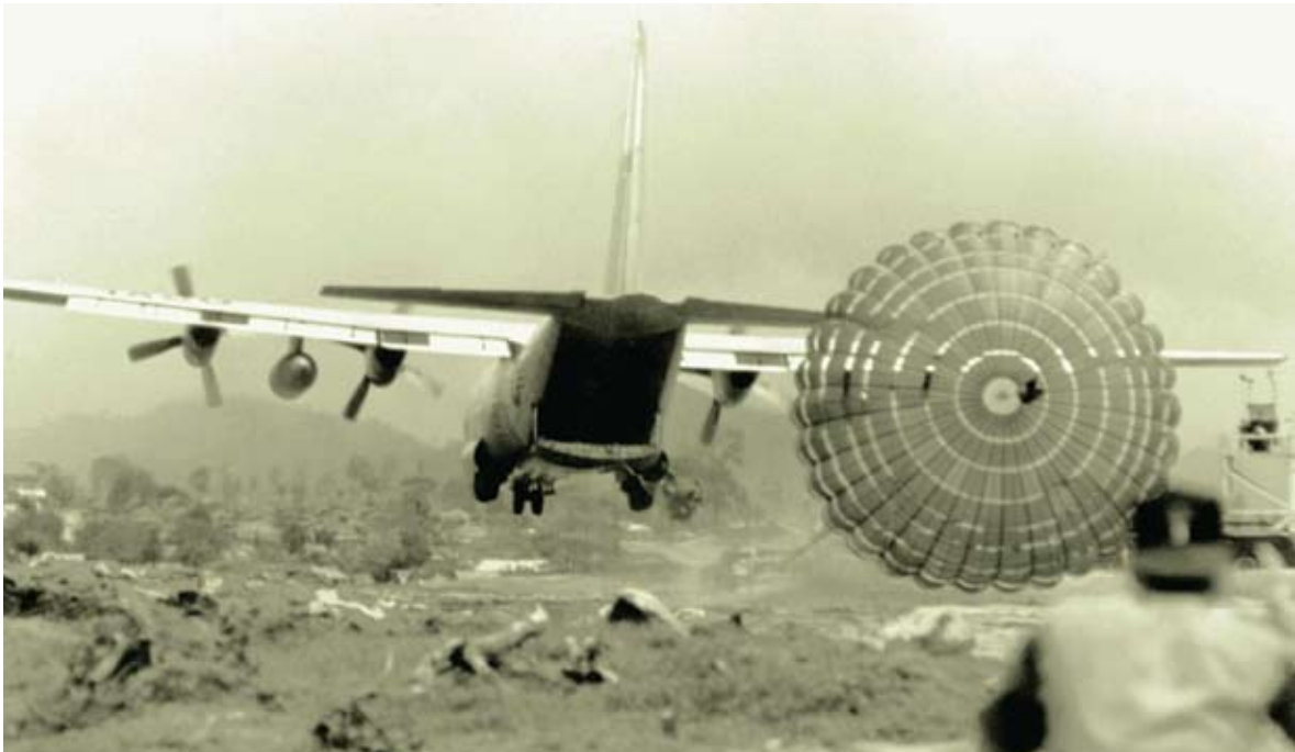
Figure 68. A C-130E making a low-altitude parachute extraction in Vietnam. (USAF photo)
