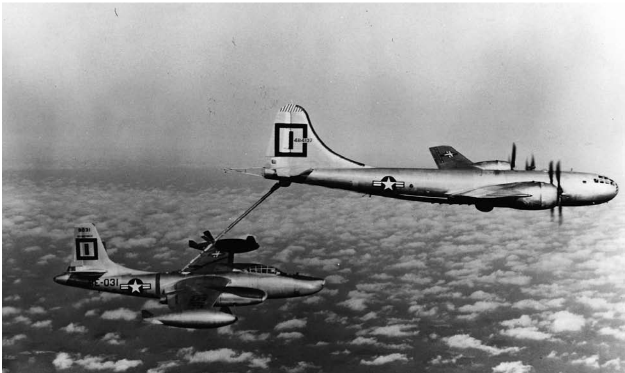
Figure 54. A KB-29 refueling a B-45. (USAF photo)
