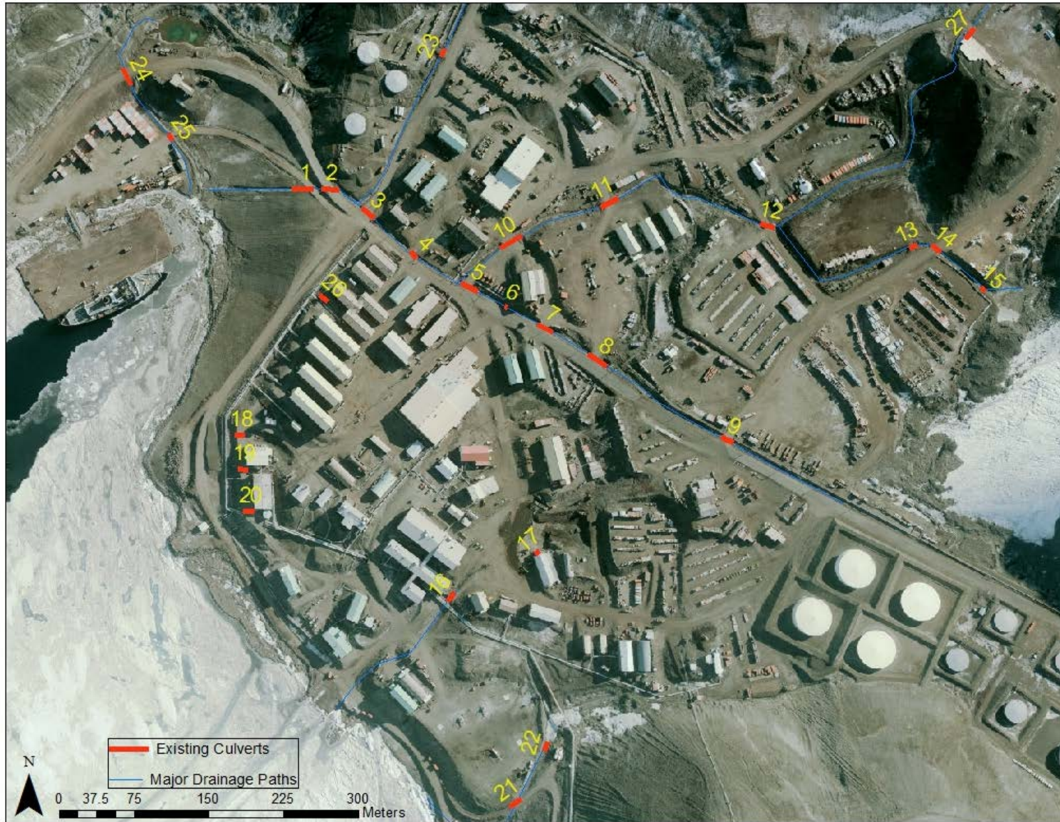
Figure 9. Existing culvert locations.
