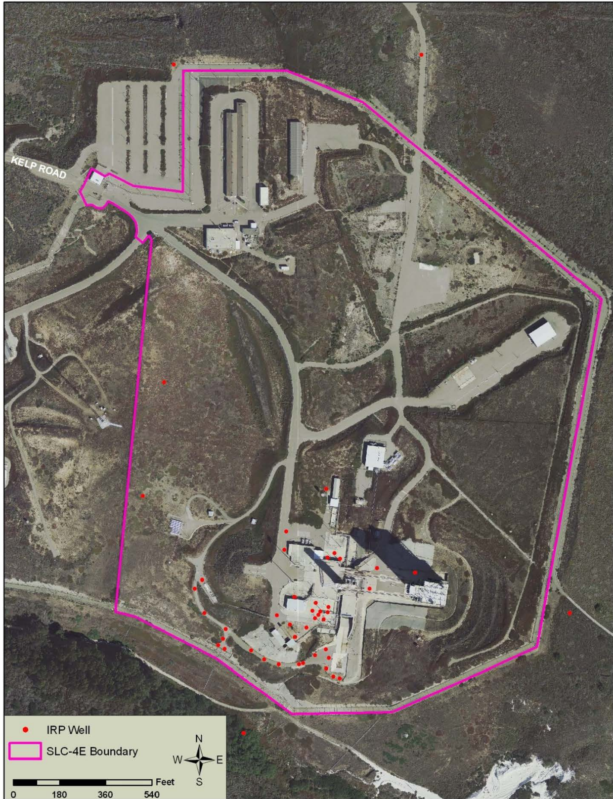
Figure 3-2. Monitoring and injections well locations at SLC-4E.
