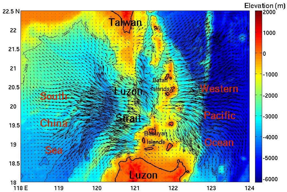
**Figure 9:** Internal wave energy flux (the largest is 10 kW/m) produced by the interaction of the M2 barotropic tides with the bathymetry in the Luzon Strait. The energy flux vectors are interpolated onto a coarse Cartesian grid from the fine unstructured grid for clarity.
