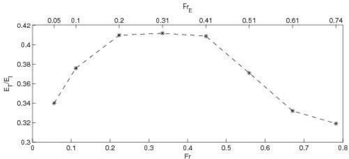
**Figure 12:** Ratio of transmitted to reflected energy for an internal wave incident on a shelf break as a function of the Froude number ( $Fr=u/c$ , where  $c$  is the internal wave phase speed and  $u$  is the maximum internal wave-induced velocity) of the incoming wave, showing how the transmitted energy peaks around  $Fr=0.3$ . The upper axis label represents  $FrE$ , the ratio of the internal wave excursion lengthscale to the topographic lengthscale.
