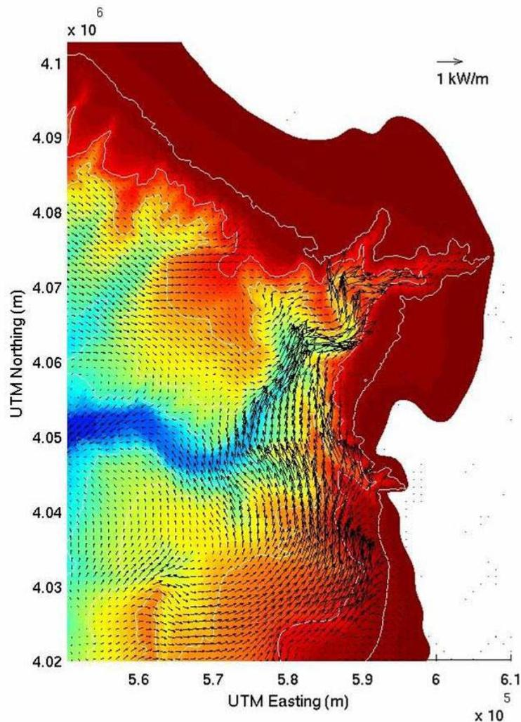
***Figure 5: Internal wave energy flux vectors in Monterey Bay, showing how a significant amount of energy is generated to the south of the Bay over Sur Platform, and this energy propagates northward into the Monterey Bay Submarine Canyon, where it is ultimately dissipated.***
