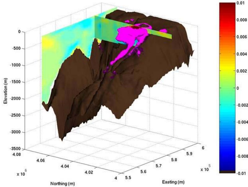
**Figure 6: Three-dimensional picture of the complex distribution of internal wave energy flux divergence in Monterey Bay. The isosurface indicates a value of  $0.003 \text{ W m}^{-3}$  while the colorbar indicates the values in the contour plots in the two transects.**
