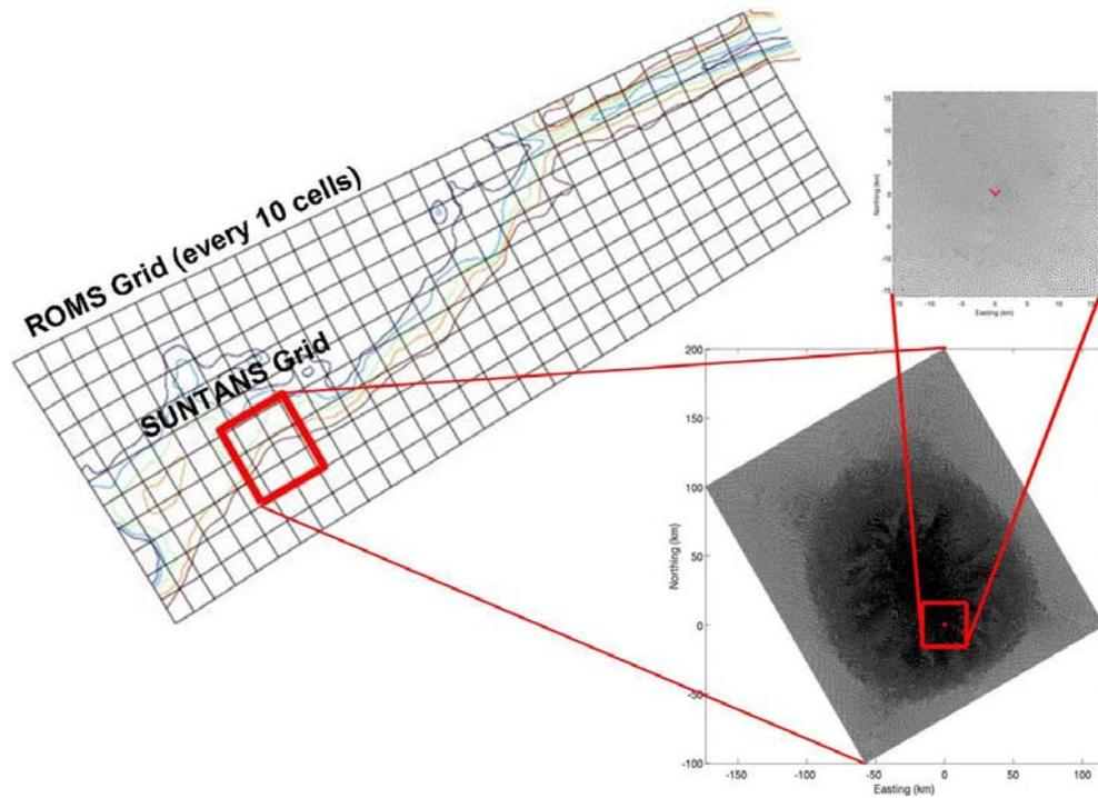
**Figure 2: Depiction of the SUNTANS grid nested within the ROMS grid, showing how a resolution of 200 m is achieved within the SUNTANS grid while the extent of the entire ROMS domain is roughly 2500 km.**
