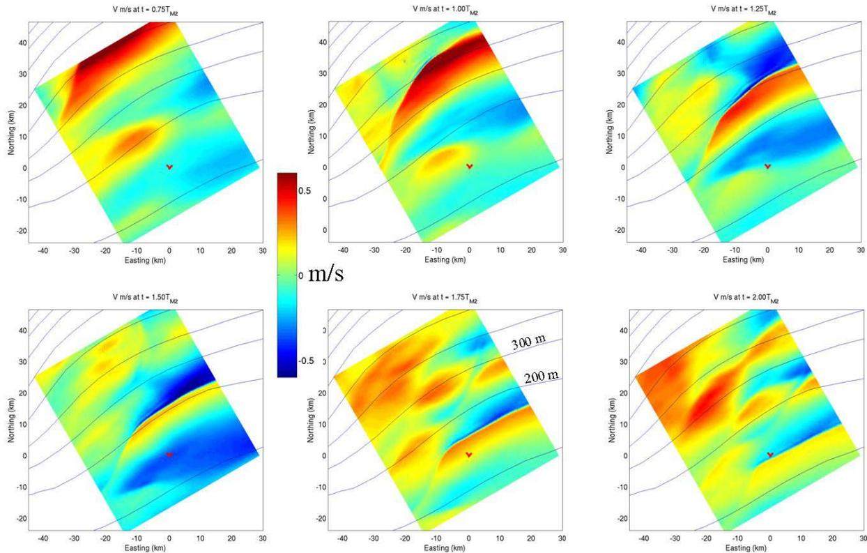
**Figure 3: Depiction of the north-south surface velocity field superimposed over depth contours (plotted every 100 m) showing the evolution of highly nonlinear internal wave fronts as they propagate southward onto the Australian North West Shelf.**
