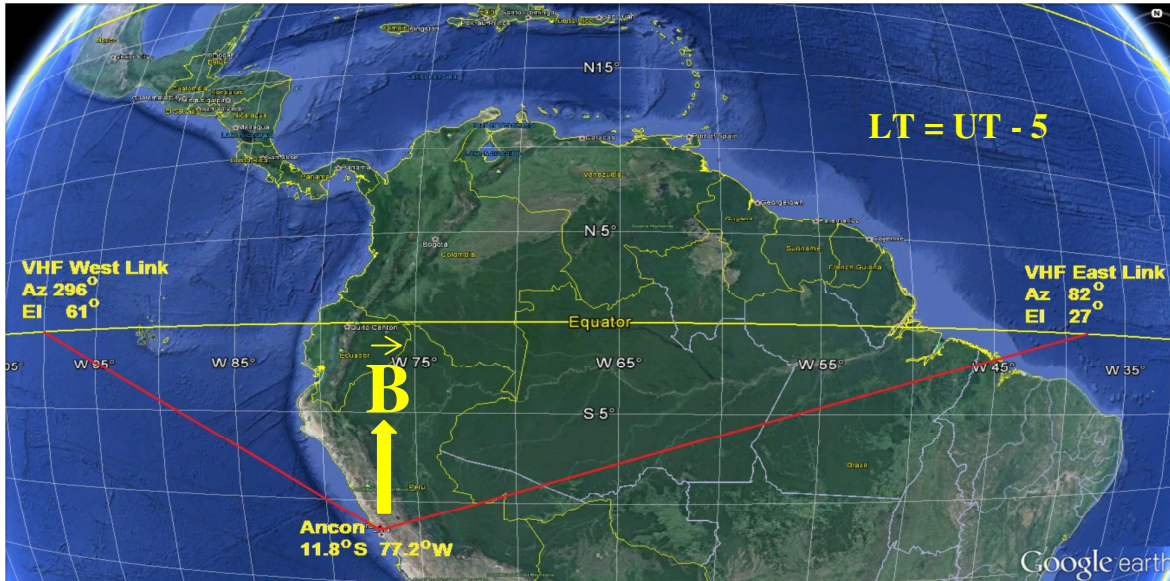
Figure 2. Projections of the West and East links from the ground receiver to geostationary satellites.
