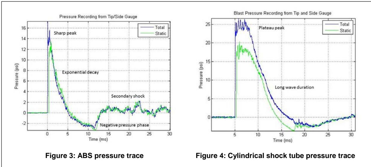
Figure 3: ABS pressure trace
