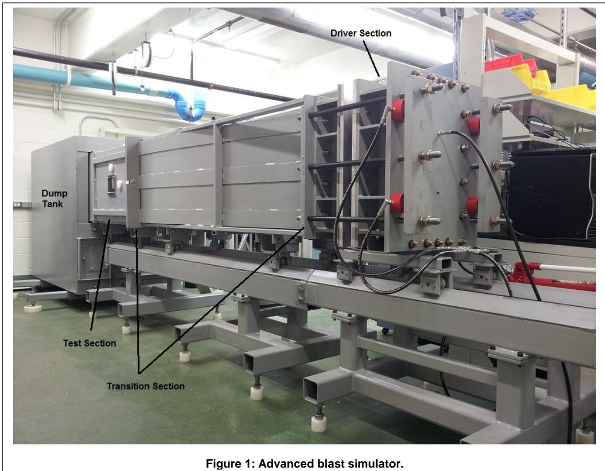
Figure 1: Advanced blast simulator.
