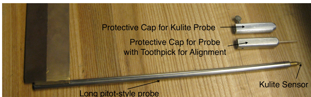
Figure 7. Long Kulite pitot probe with alignment cap and protective cap.
