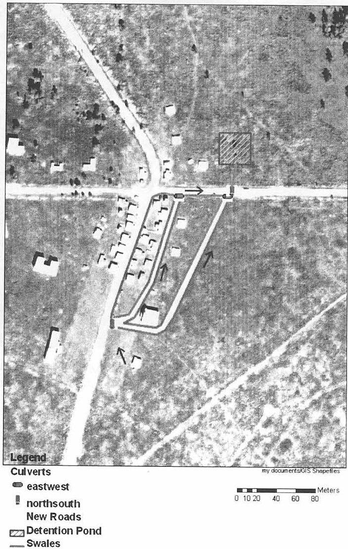
Figure 3. Aerial view of North MOUT showing locations of new roads, swales, culverts, and detention pond.
