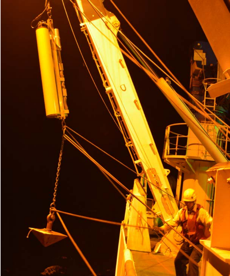
Figure 51. Lowered source deployment.
