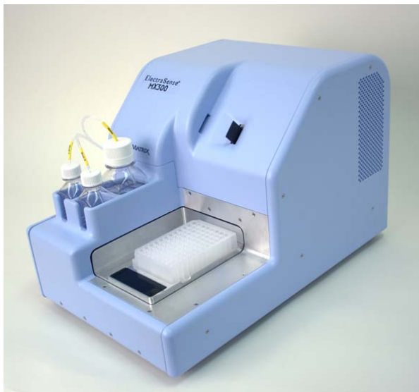
Figure 2. ElectraSense MX300 automated chip reading/washing station. Fully automated, contains four fluid control lines for applying four samples to the same chip. Serial address chip interface for voltage/current readout.
