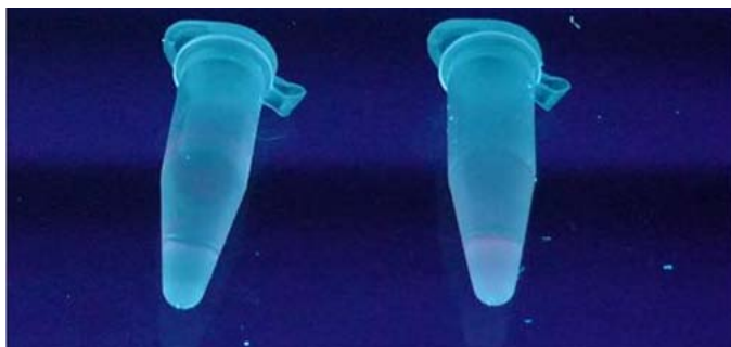
Figure 8. Vial containing S. typhimurium beacon in quenched state before target added (left) and beacon in unquenched state after addition of 1 mM target sequence (right). The decrease in photoluminescence is visible by the naked eye.
