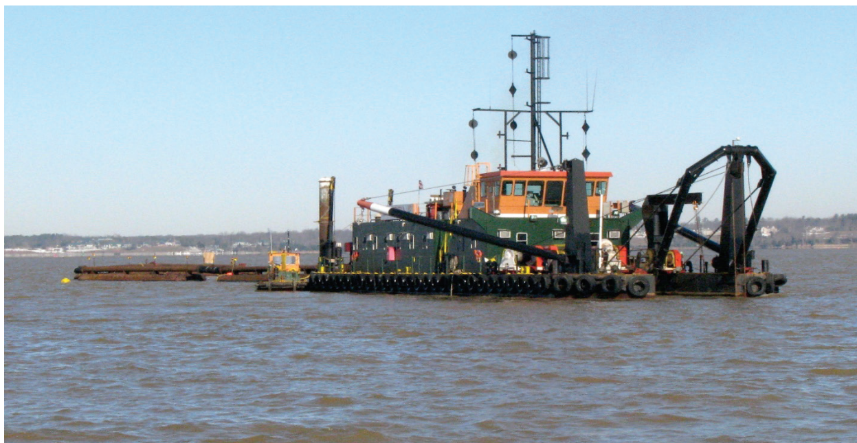
Figure 2. The hydraulic cutterhead dredge Lexington operating in the James River, Virginia.
